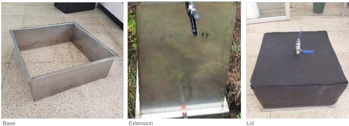
Figure 3. Static chamber for field GHG measurements in Ecuador.
